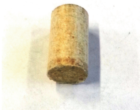
Figure 5. Example of the ‘oil gradient’ in L 1 pellet produced at 150 MPa.
