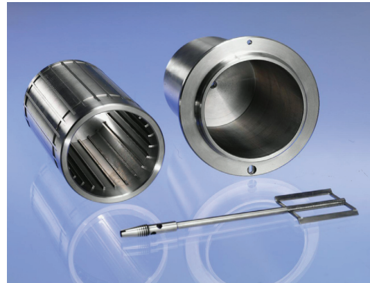
Figure 2. Measuring cell and vane rotor for the determination of the rheological properties of pastes and mortars with a Thermo Scientific HAAKE Rheometer.
