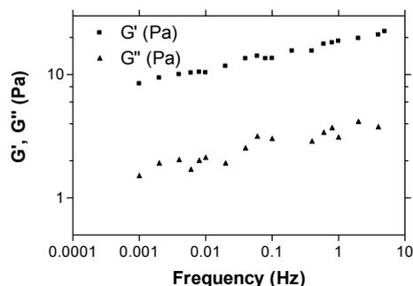
Figure 1. Frequency sweep of salmon skin mucus over the frequency range 0.001-5 Hz showing the elastic modulus ( $G'$ ) and the viscous modulus ( $G''$ ).
