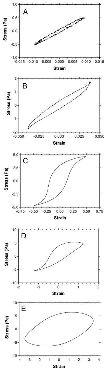
Figure 4. Lissajous figures showing the relationship between stress and strain during single oscillatory cycles of the strain sweep at 1Hz, for reference the measured phase angles for the data points were 6.0° (A), 7.5° (B), 18.1° (C), 17.2° (D) and 25.5° (E)
