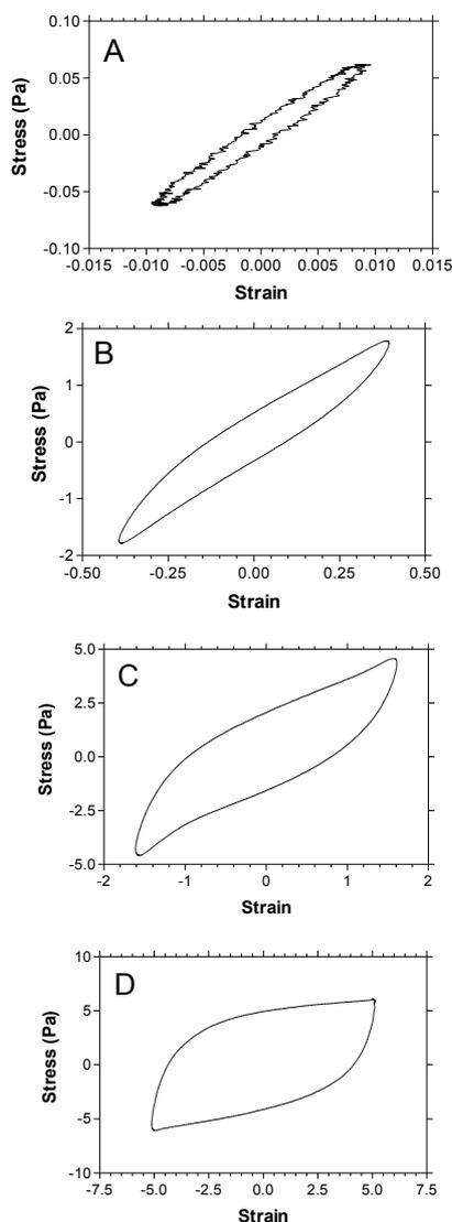
Figure 3. Lissajous figures showing the relationship between stress and strain during single oscillatory cycles of the strain sweep at 0.1 Hz, for reference the measured phase angles for the data points were  $10.1^\circ$  (A),  $13.6^\circ$  (B),  $22.1^\circ$  (C) and  $43^\circ$  (D)
