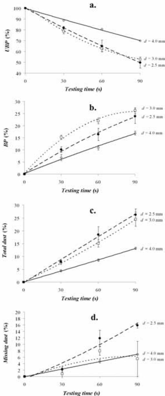
Figure 6. Averages ( $n = 3$ ) of *UBP (%)*, *BP (%)*, *Total dust (%)* and *Missing dust (%)*, in the Holmen tester for three different types of pelleted feed. The error bars represent the standard error of the mean.
