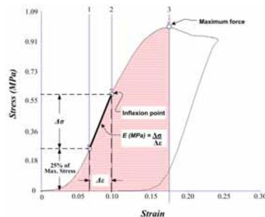
Figure 7. Texture profile analysis of one of the pellets ( $d = 4$  mm) having a ductile behaviour.
