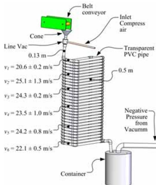
Figure 3. Assembly used to simulate pneumatic transport conditions. This system will be used to evaluate the principle of a potential new pellet tester. The figure shows averages of air speed ( $v$ )  $\pm$  the standard error of the mean ( $n = 3$ ).
