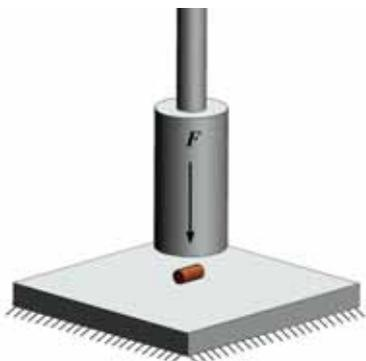
Figure 4. Diametrical compression of a feed pellet using a cylindrical probe, SMS P/45.
