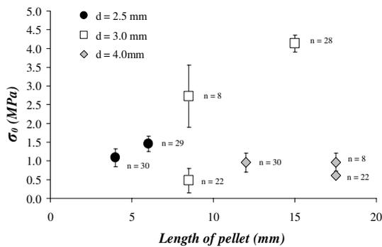
Figure 8. Maximum tensile stress that produces failure in 63.2% of the pellets. Stresses from three different types of pelleted feed having three different diameters are shown. The error bars represent the CV that was estimated through the Weibull modulus.
