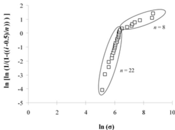
Figure 9. Weibull probability plot for the 3.0 mm pellets having a length of 8.5 mm.
