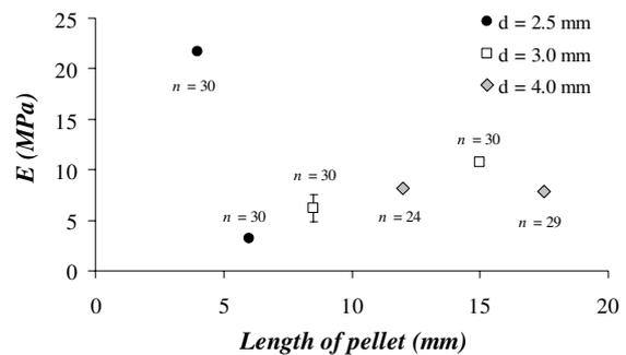
Figure 10.  $E$  for three different types of pelleted feed having three different diameters. Each feed was separated in two groups of different lengths. The error bars represents the CV.
