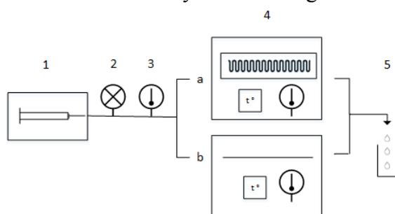
Figure 2. The experimental arrangement: 1 – linear pump, 2 – pressure sensor, 3 – temperature sensor, 4a – microfluidic reactor, 4b – capillary, 5 – product collection and sampling.
