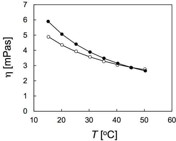
Figure 3. Temperature dependencies of viscosity of binary (o) and ternary (•) mixtures.
