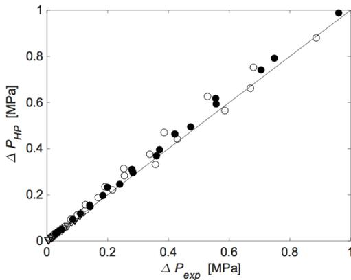
Figure 4. Predicted vs. measured pressure drop in capillary: methanol (▼), binary (o) and ternary (•) mixtures. A diagonal guides eyes to  $\Delta P_{HP} = \Delta P_{exp}$ .
