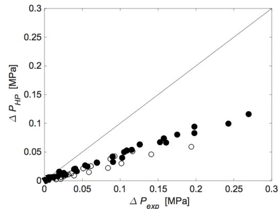
Figure 5. Predicted vs. measured pressure drop in microreactor: methanol (▼), binary (o) and ternary (•) mixtures. A diagonal guides eyes to  $\Delta P_{HP} = \Delta P_{exp}$ .
