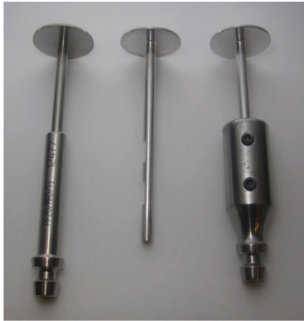
Figure 2. Different geometries used in measurements. Anton Paar geometry left, custom made geometries with and without adapter.
