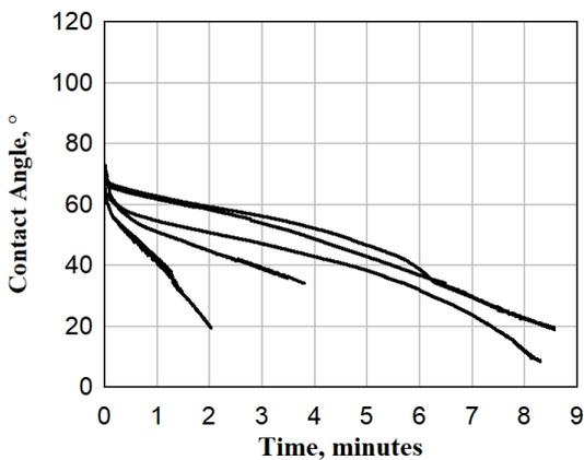
Figure 12. Wettability of coated pellets using 2 minutes of pressure release.
