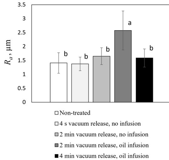
Figure 5. Average surface roughness,  $R_a$ , for non treated and vacuum treated pellets. Pressure changes were applied with and without oil.
