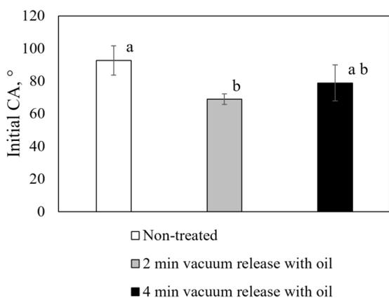
Figure 10. Initial contact angle. Means ± CI that do not share a letter are significantly different ( $p < 0.05$ ).
