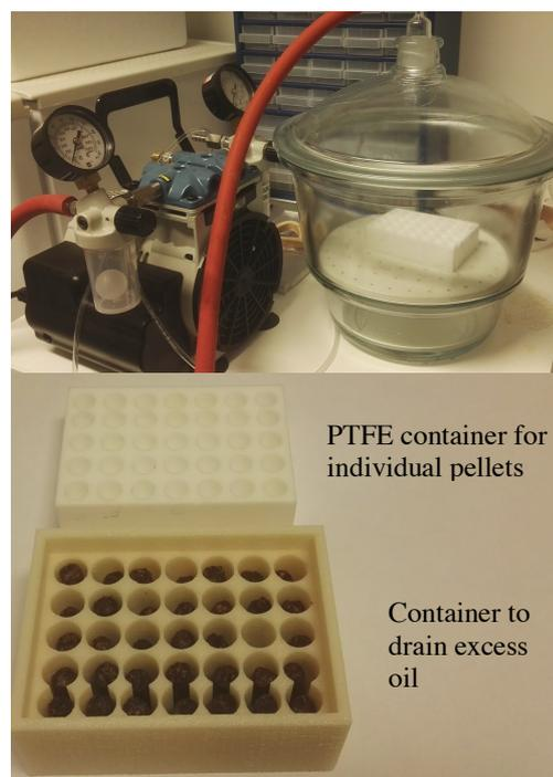
Figure 1. Arrangement to infuse oil through vacuum. The top picture shows a glass vacuum chamber having a PTFE container inside. The chamber is connected to a vacuum pump. At the bottom, a detailed view of the PTFE container and a container to drain the excess oil.
