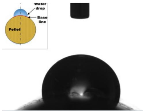
Figure 4. Example of a drop profile extraction and the measurements of contact angle on a cylindrical surface of a pellet. Image taken from Misljenovic et al.<sup>6</sup>
