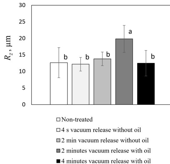
Figure 6. Mean peak-to-valley height,  $R_z$ , for non treated and vacuum treated pellets. Pressure changes were applied with and without oil.
