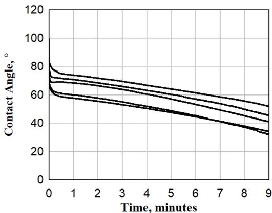
Figure 13. Wettability of coated pellets using 4 minutes of pressure release.
