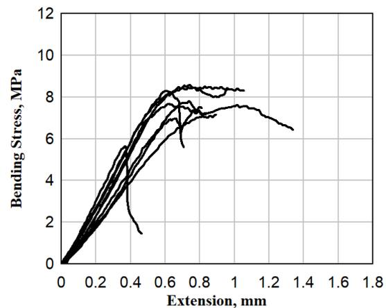
Figure 9. Bending stress (MPa) of coated pellets using 4 minutes pressure release time.
