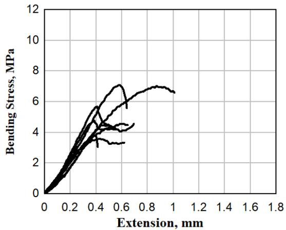
Figure 8. Bending stress (MPa) of coated pellets using 2 minutes pressure release time
