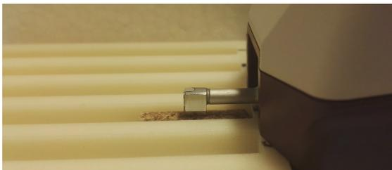
Figure 2. Needle profiler measuring the surface roughness of a pellet
