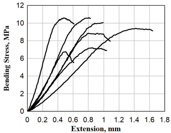
Figure 7. Bending stress (MPa) of un-treated wood pellets
