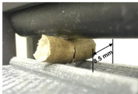
Figure 3. Three-point bending test. The picture shows a pellet fracture during testing. Image taken from Misljenovic et al.<sup>6</sup>
