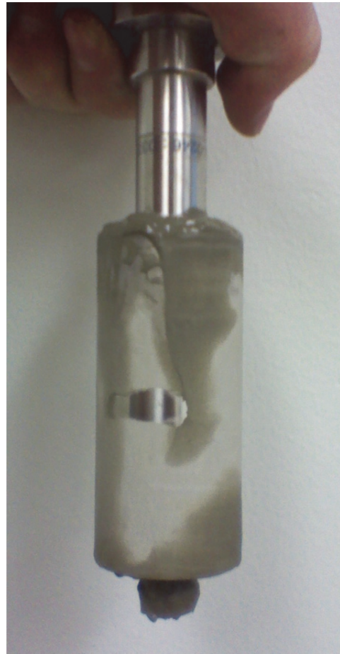
Figure 5. The bob of the MARS rheometer after it has been removed from the pressure cell after measurement at elevated temperature over one hour.
