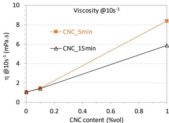
Figure 3. Influence of CNC content on viscosity of water as measured at  $10\text{s}^{-1}$  for different mechanical dispersion times.
