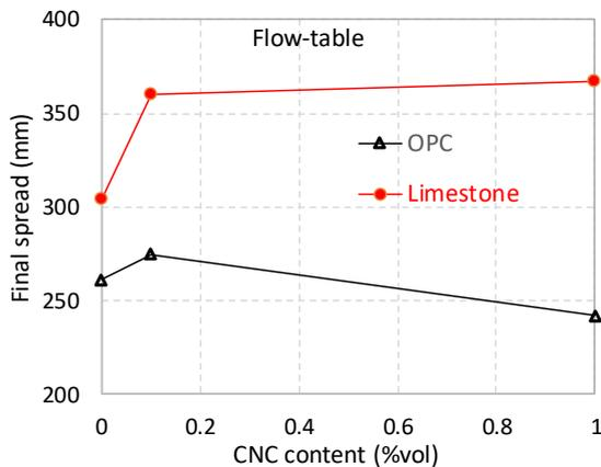
Figure 7. Flow-table results of mortars prepared with Limestone and OPC as a function of CNC content.
