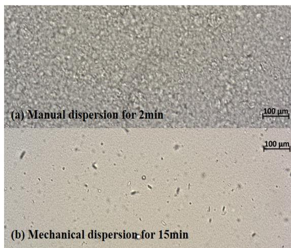
Figure 2. Optical microscopy images of CNC dispersion in water: (a) manual dispersion for 2min; (b) mechanical dispersion for 15min.
