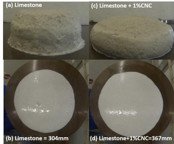
Figure 8. Flow-table images of mortar prepared with Limestone. (a), (b) 0%CNC; (c), (d) 1%CNC. (a), (c) before the test; (b), (d) after the test.
