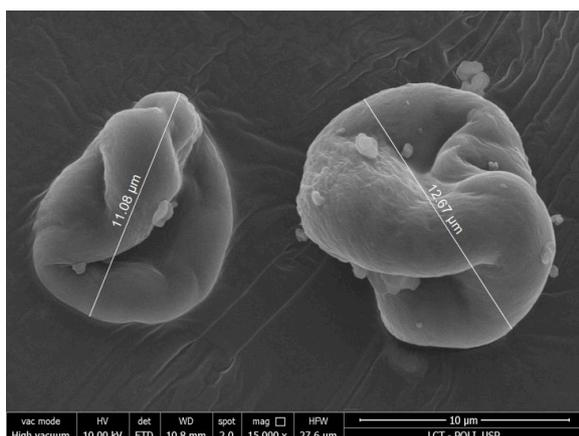
Figure 1. SEM image of dry CNC particles.
