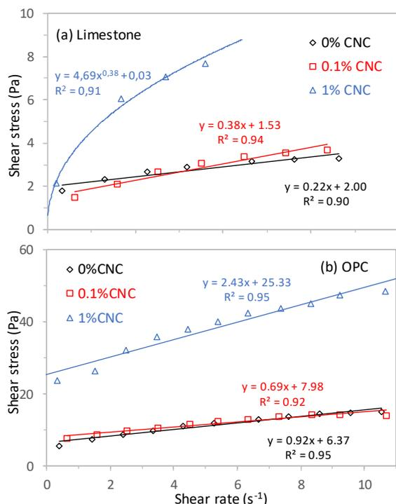
Figure 5. Rotational rheometry results of (a) Limestone and (b) OPC suspensions in function of CNC content.
