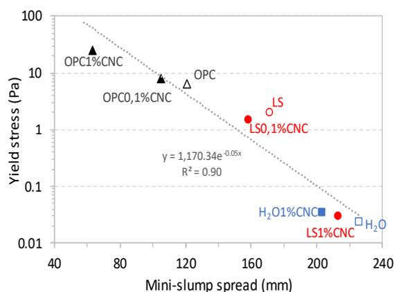
Figure 6. Yield stress as determined by rotational rheometry vs. spread diameter obtained in the mini-slump test. LS = Limestone; OPC = Cement; H<sub>2</sub>O = water.
