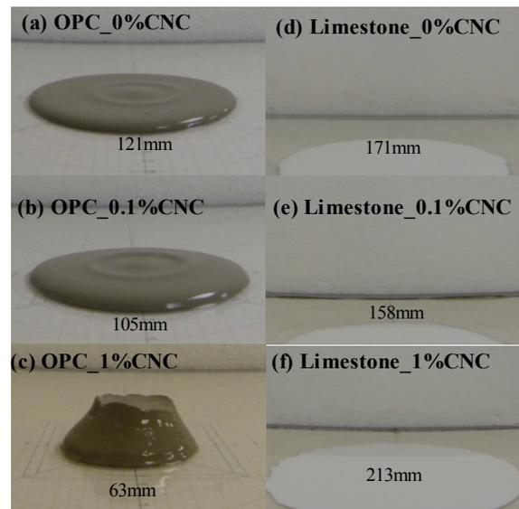
Figure 4. Mini-slump images and results of OPC and limestone suspensions in function of CNC content.
