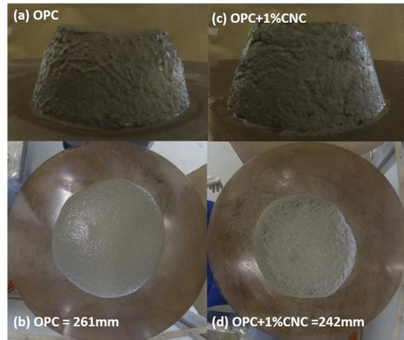
Figure 9. Flow-table images of mortar prepared with OPC. (a), (b) 0%CNC; (c), (d) 1%CNC. (a), (c) before the test; (b), (d) after the test.
