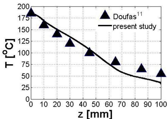
Figure 6. Comparison of the film temperature with the experimental result in the literature<sup>11</sup>,  $D_R=10$ ,  $\Delta P=0.0015$  XPP model
