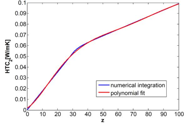
Figure 2. Fitting of the heat transfer coefficient for the free film surfaces, numerical integration of the coefficient in the literature<sup>11</sup>, the 7<sup>th</sup> order polynomial fit used in this study
