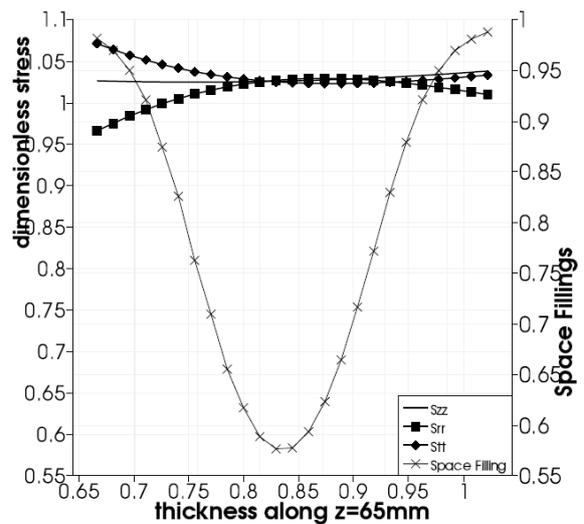
Figure 5. Dimensionless stresses and space filling distributions along the thickness at  $z=65$ mm,  $D_R=10$ ,  $\Delta P=0.0015$  XPP model
