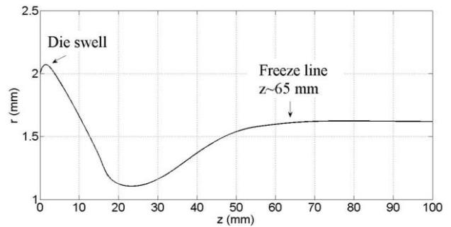
Figure 4. Bubble shape,  $D_R=10$ ,  $\Delta P=0.0015$  XPP model
