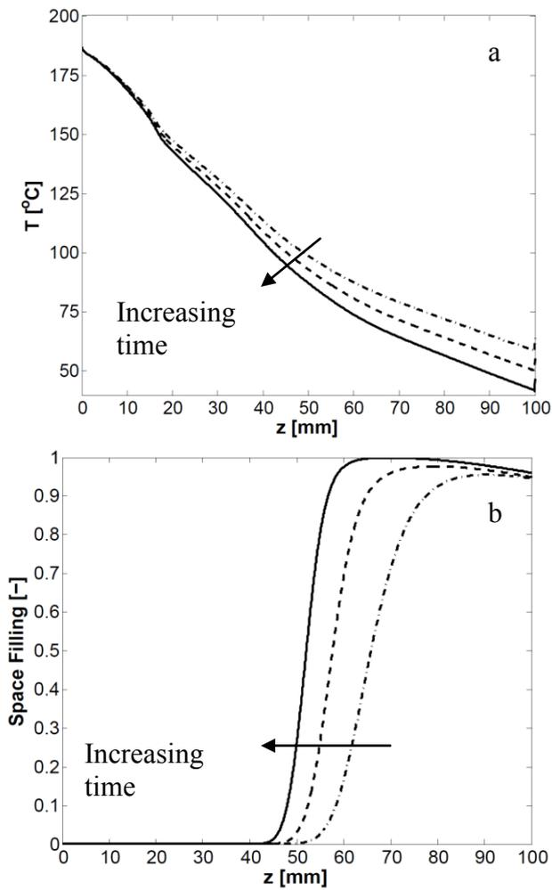
Figure 3. (a) Temperature distribution evolution along the outer film surface (b) space filling distribution evolution along the outer film surface,  $D_R=10$ ,  $\Delta P=0.0015$  XPP model
