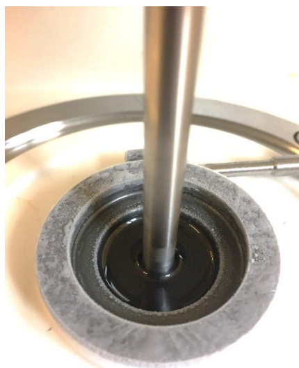
Figure 3. Soy sauce at sub-zero temperature in the CC27 bob/cup system. A thin oil layer is placed on surface of the sauce to prevent dilution from water originating from the surrounding air.
