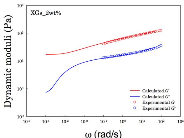
Figure 2. Comparison of measured and calculated dynamic moduli of XGs 2wt%.
