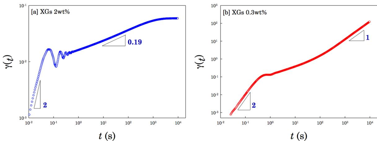
Figure 1. Creep ringing of xanthan gum solution (0.3wt% and 2wt%)
