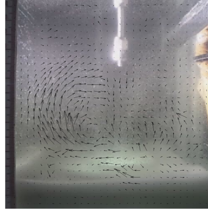
Figure 11: Superposition of cropped picture of the velocity vectors averaged from 300 images.
