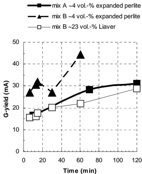
Figure 4. Effect of light-weight aggregate on G-yield
