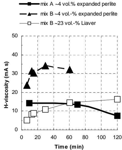
Figure 5. Effect of light-weight aggregate on H-viscosity
