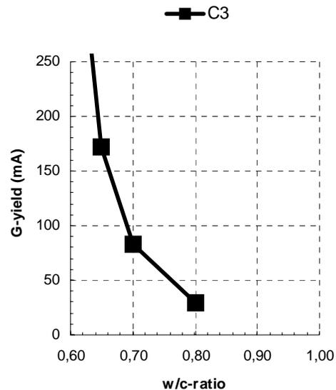
Figure 3. Effect of w/c-ratio on rheology
