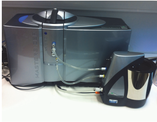
Figure 3. Milk sample in the Malvern Mastersizer 3000 using the Hydro LV dispersion unit.
