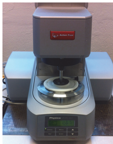
Figure 1. Milk sample measured by rotational viscometry using a Physica MCR 301 rheometer with a bob/cup measuring geometry.
