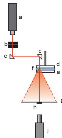
Figure 1: Arrangement for the Rheo-SALS experiments: (a) He–Ne laser; (b) aperture and neutral density filter; (c) prisms; (d) rotating glass plate; (e) base plate containing circulating heating/cooling water and glass window; (g) translucent screen; (h) beam stop; (j) CCD camera
