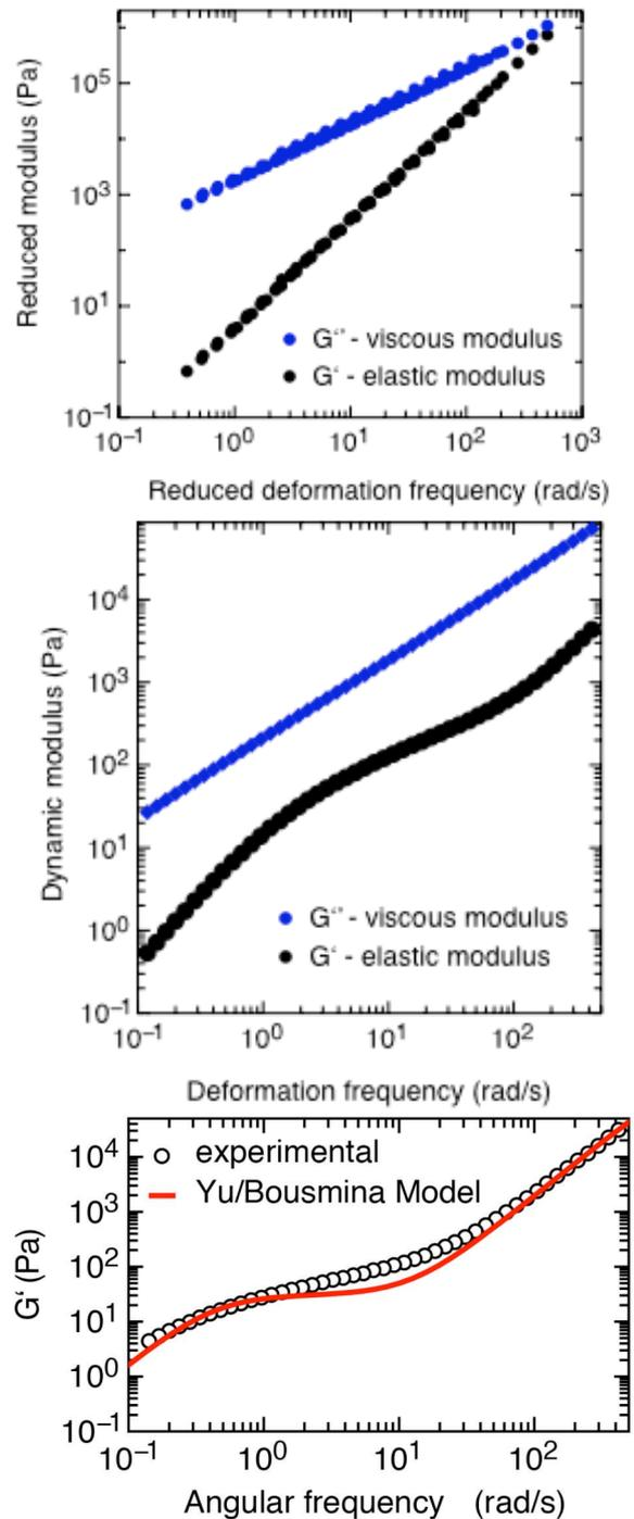
Figure 3: Frequency-dependent dynamic moduli of emulsions with dominant shape relaxation stabilized by excess SDS. (a) Reduced storage and loss moduli,  $G'$  and  $G''$ , of the continuous phase. (b)  $G'$  and  $G''$  at 20°C of an emulsion prepared with SDS (oil phase fraction  $\phi = 4.5$  vol.%). The arrow indicates the characteristic relaxation shoulder of the storage modulus, caused by shape relaxation of the deformed
