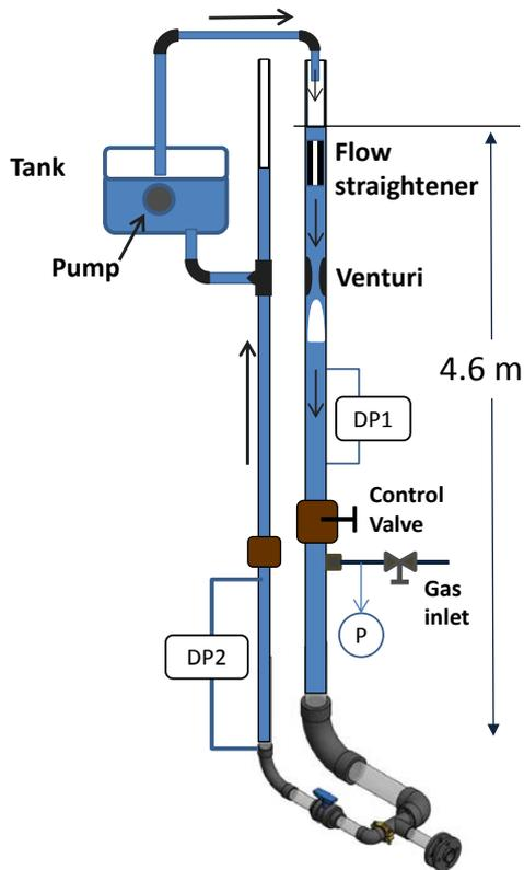
Figure 4: Experimental setup of the flow rig
