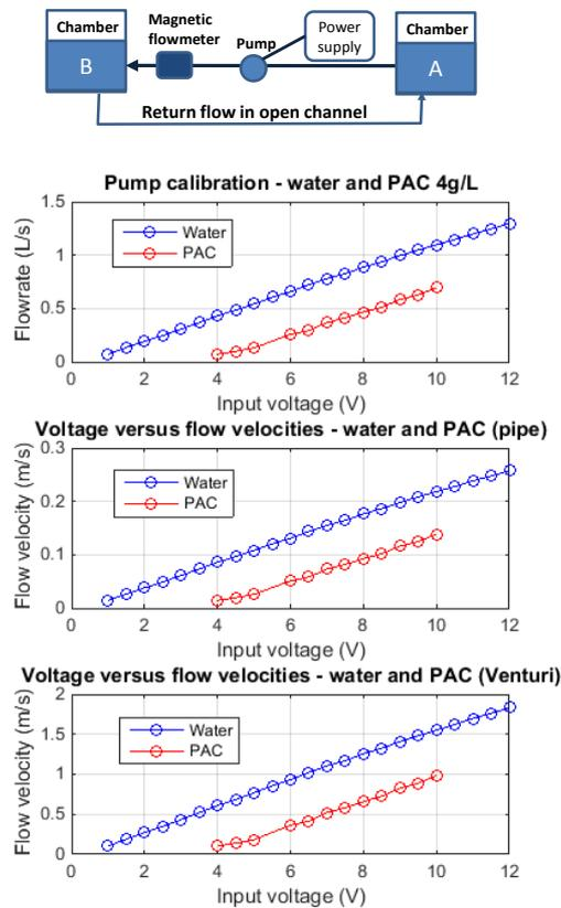
Figure 7: Pump calibration for water and PAC. Pump flow rate and velocity in the pipe and in the Venturi throat as a function of voltage.
