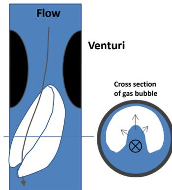
Figure 13: The bubble is shifted and deformed by the asymmetric velocity profile which “self-organizes” with the bubble
