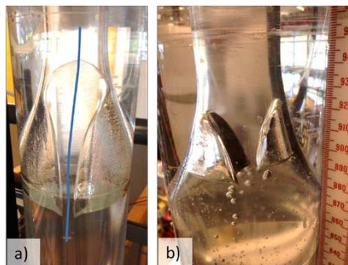
Figure 12: a) PAC 4 g/L bubble seen into the deep split at 12V pump power. The flow direction is indicated by the long arrow. The bubble may eventually be cut into two pieces b) A similar distribution often arises when air is injected from the top. It then flows down as smaller bubbles from the top and coalesce into larger bubbles in the wake.
