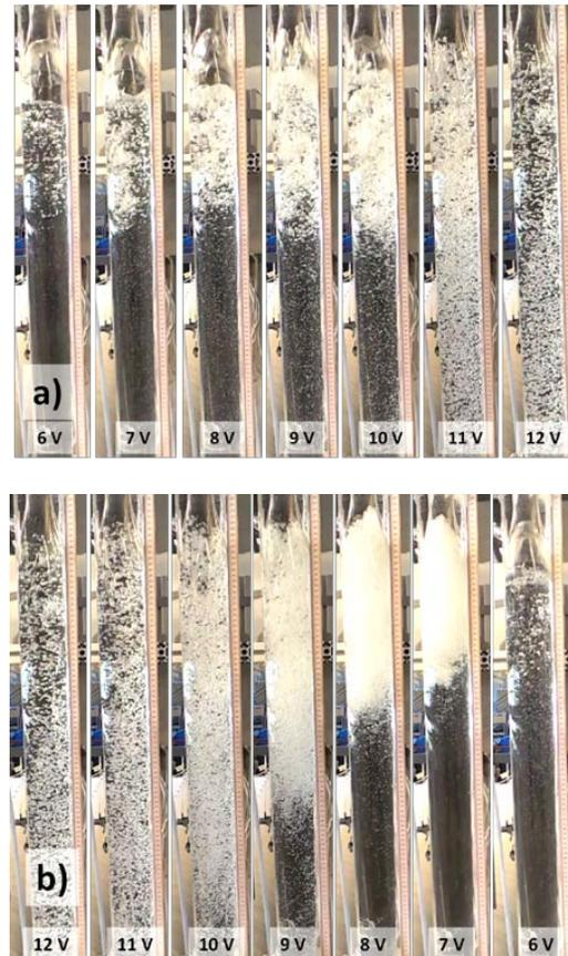
Figure 8: Bubble breakup process in water experiments for a) increasing flowrate (6-12 V) and in b) decreasing flowrate (12-6 V)
