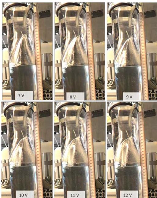
Figure 10: For PAC 3g/L the big bubble does not break but is more and more distorted for voltage/flowrate (6-12 V).
