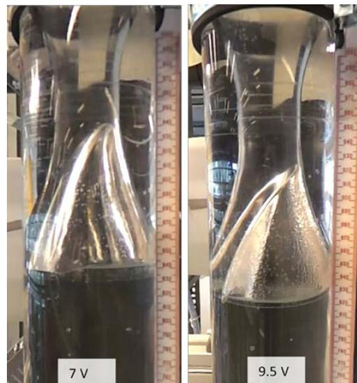
Figure 11: For PAC 4 g/L the big bubble does not break but is more and more distorted for voltage/flowrate (6-12 V).
