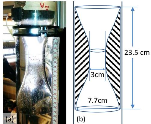
Figure 5: The Venturi placed inside the pipe. a) Picture b) Drawing and dimensions
