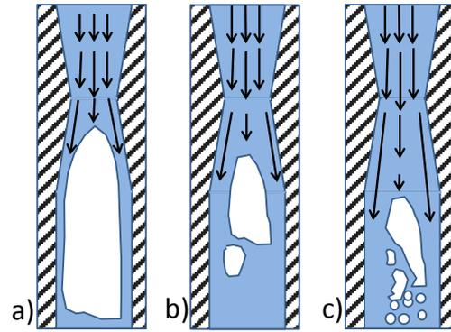
Figure 2: A large gas bubble trapped in a divergent expanding pipe flow field. The position of the bubble is self-regulating for a fixed liquid flow rate.
