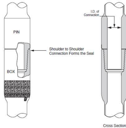
Figure 1: Tool joint parts of the drillstring makes contractions similar to Venturis.
