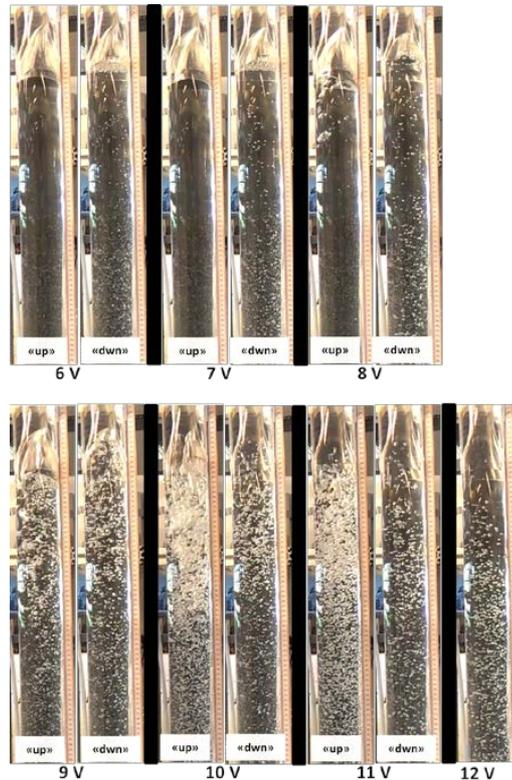
Figure 9: Breakup process for PAC 1g/L. Voltage/flowrate (6-12 V) arranged as pairs for increase (up) and decrease (dwn).
