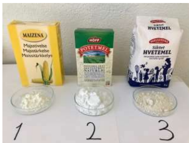
Figure 1: The three different starch containing sources used in this rheological investigation; 1 Maize, 2 Potato, 3 Wheat.
