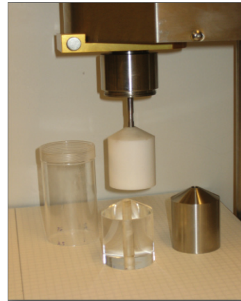
Figure 1. Rotor and stators in acrylic and teflon together with original stainless steel stator.
